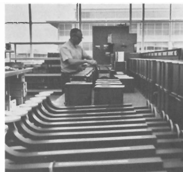
Richard Sermol works behind line of waveguide directional couplers.
