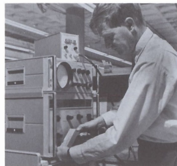
Spectrum analyzer helps Rod Carlson check new frequency comb generator.
